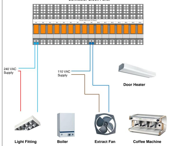
Use any TYPE of Appliance up to 16 amps as Standard or if you need higher amps or 3 phase, use an additional relay.
