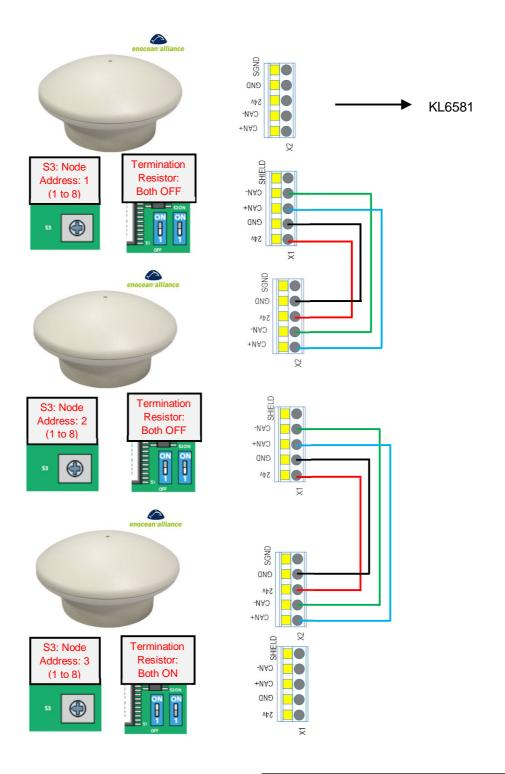
Maximum 8 Domes per line. Cable total length 500m. Daisy chain, NOT star wiring.
