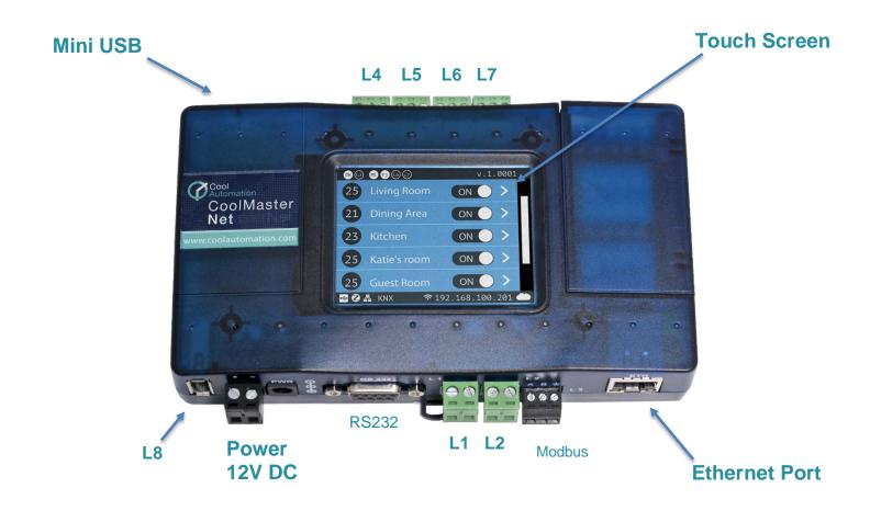
Air Conditioning Communication Bus Lines: L1 – L2: For Mitsubishi Electric, Daikin, Toshiba, Panasonic, Sanyo and Hitachi L4 – L7: For Mitsubishi Heavy Industries, LG, Samsung, and Gree L8 – USB Port for Echelon Stick - Fujitsu רמ"ד
